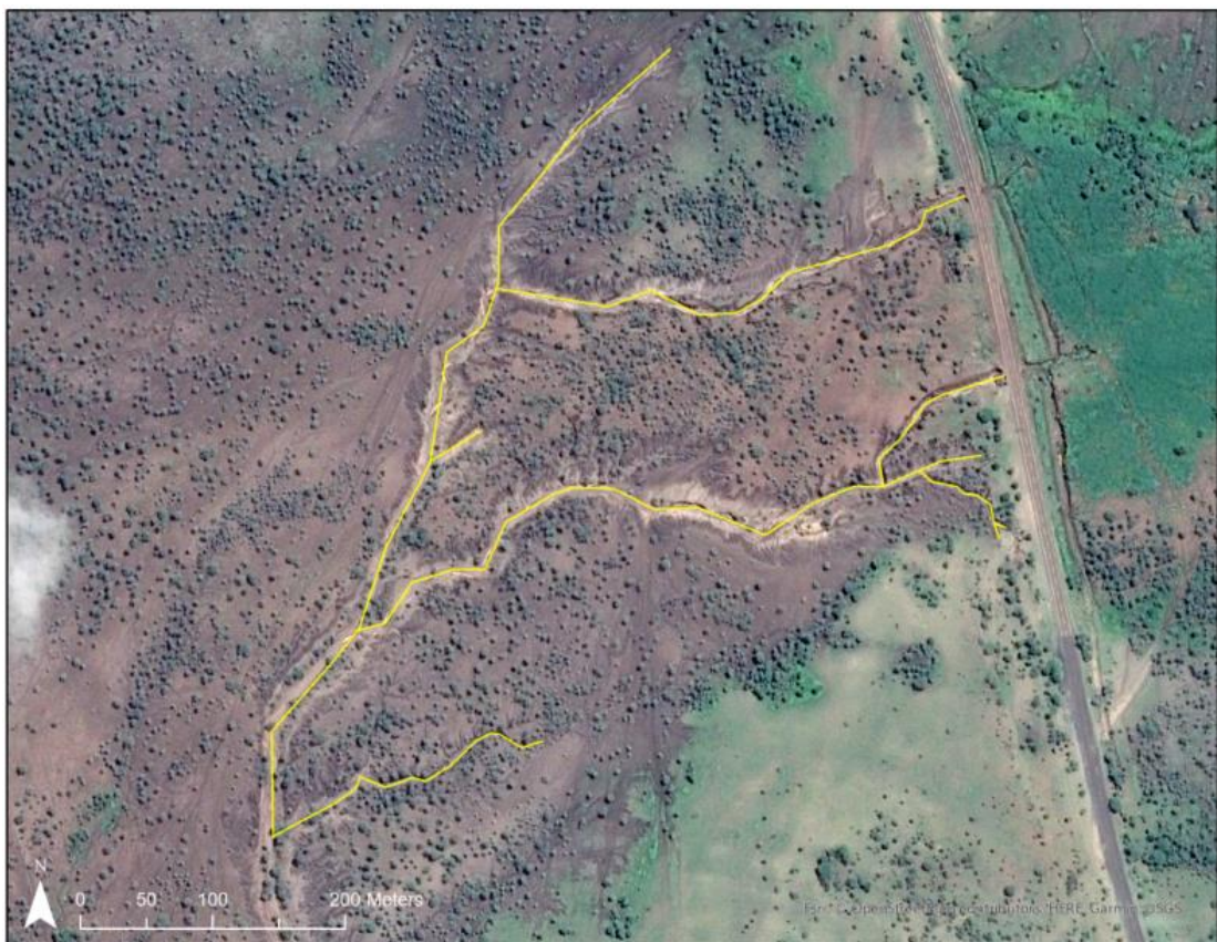
Figure 7: Google Earth Pro image (CNES/Airbus) of 13-03-2017 adapted with line segments in ArcGis Pro. Length of this part of the gully is 2154.9 meters
