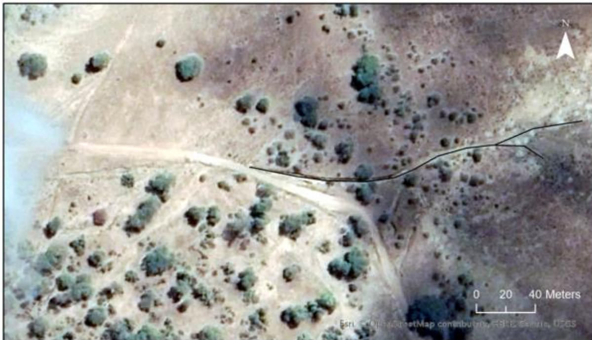
Figure 11: Google Earth Pro image (CNES/Airbus) of 26-08-2019 adapted with line segments in ArcGis Pro. Length of this part of the gully is approximately 302.4 meters
