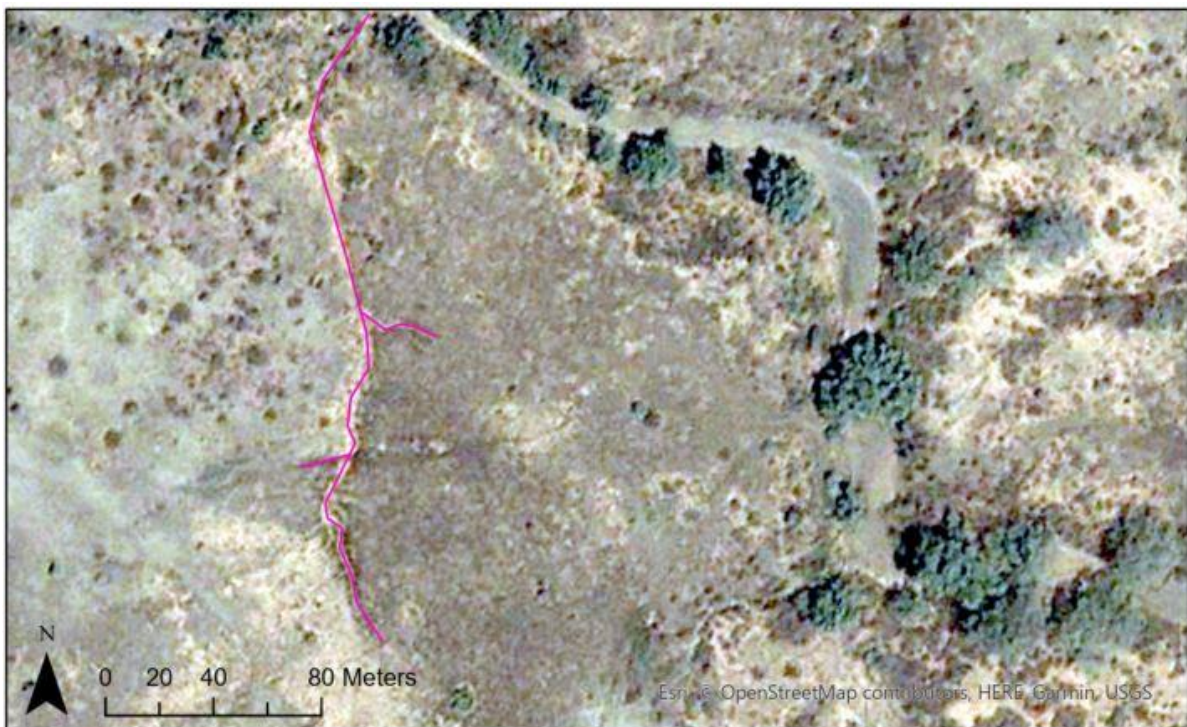
Figure 8: Google Earth Pro image (IKONOS) of 12-09-2005 adapted with line segments in ArcGis Pro. Length of this part of the gully is approximately 302.4 meters
