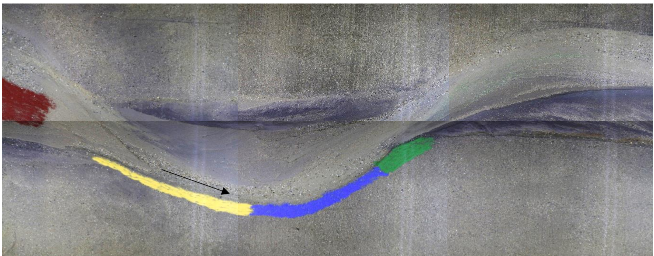
Figure 4.3 – At bend 1 colored particles were added to the outer bend in order to determine where eroded sediment deposits. The black arrow indicates flow direction.
