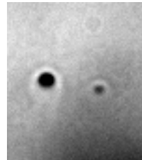
Figure 4.7: An broken bead next to a normal one for comparison.
