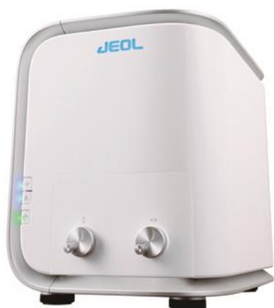
Figure 4.2. The JEOL JCM-6000 NeoScope Benchtop SEM used for analyses of thin sections P58b.
