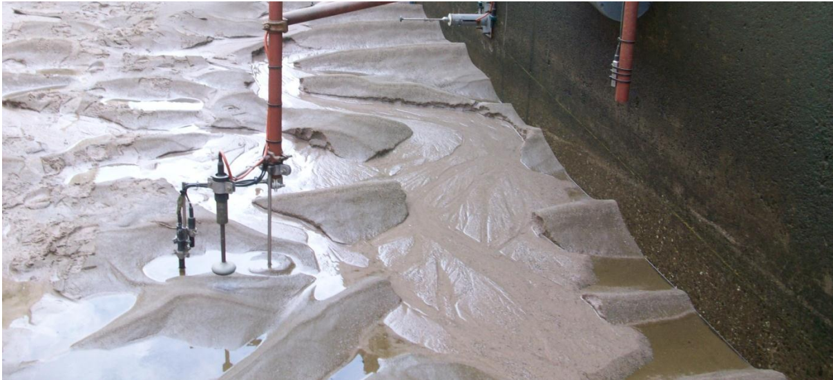
Figure 34: Large ripples around measuring instruments.
