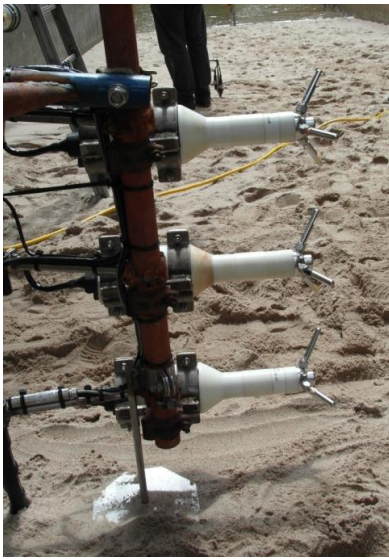
Figure 14: Measuring instruments. (a) pressure transducer (PT), (b) right: electromagnetic flow meter (EMF) and left: optical backscatter sensors (OBS), (c) acoustic Doppler velocimeters (ADV), and (d) sonar 3D scanner. Pictures: Daan Wesselman.
