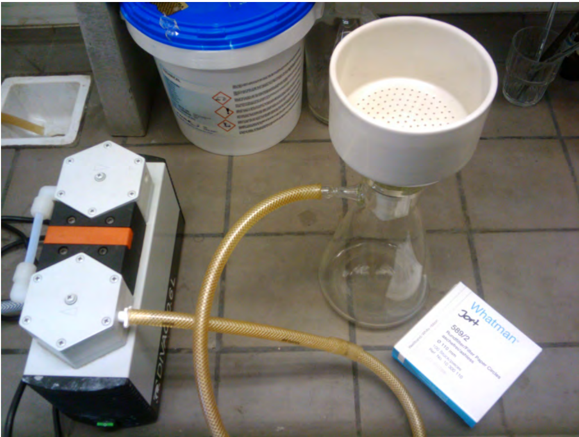
Figure A2.1. Büchner funnel setup with vacuum pump.
