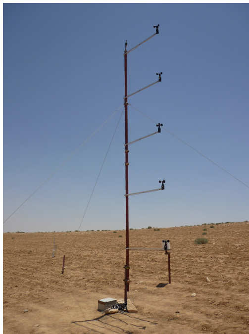
Figure 3.1: Wind tower with 5 Anemometers and one wind direction sensor at the top.
