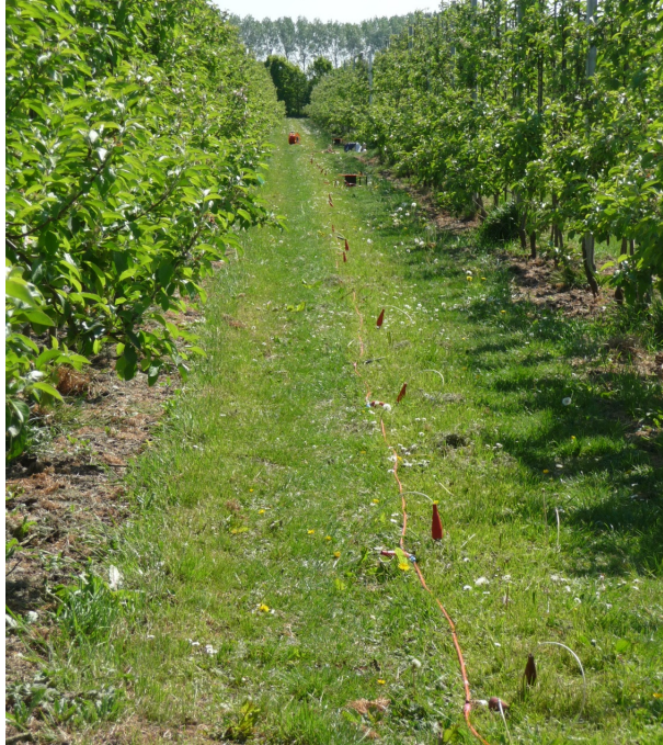
Figure 7: CVES equipment in the field in Walcheren. Electrodes are pushed into the ground every metre along the transect, and are controlled automatically by a unit seen in the distance.
