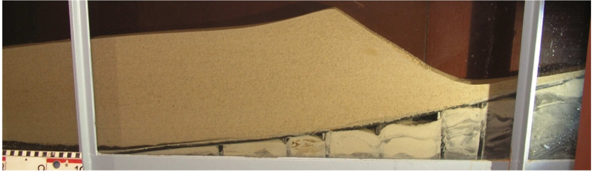
FIGURE 39: PHOTOGRAPH OF THE DEPOSITS OF RUN 12 WITH SCALE IN CMS. THE DEPOSIT IS LAMINATED THROUGHOUT.
