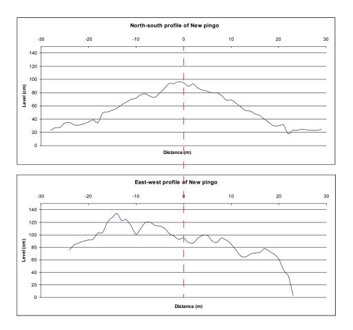
Figure 4.4: Elevation profile of the New pingo, Illisarvik, Canada
