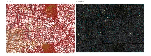
Figure 4.40: The result of depression recognition with (A) ArcGIS and (B) eCognition on the test area
