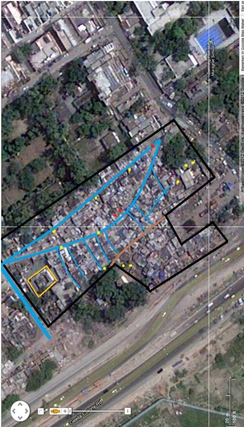
Figure 3: Map of Safeda Wali Jhugi in Geeta Colony. Black lines: borders of the colony. Blue lines: water pipe lines. Red dots: main water collection points. Yellow dots: hand pumps. Yellow square: public toilets. Brown line: Border of area with pipe water supply.
