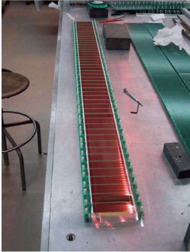
Figure 8: A single strip of the ALICE TOF detector [1]
