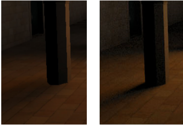
Figure 5.4.5: Loss of shadow detail using imperfect shadow maps, images extracted taken from [36]. The left image is rendered using imperfect shadow maps, the right image is a path traced reference.
