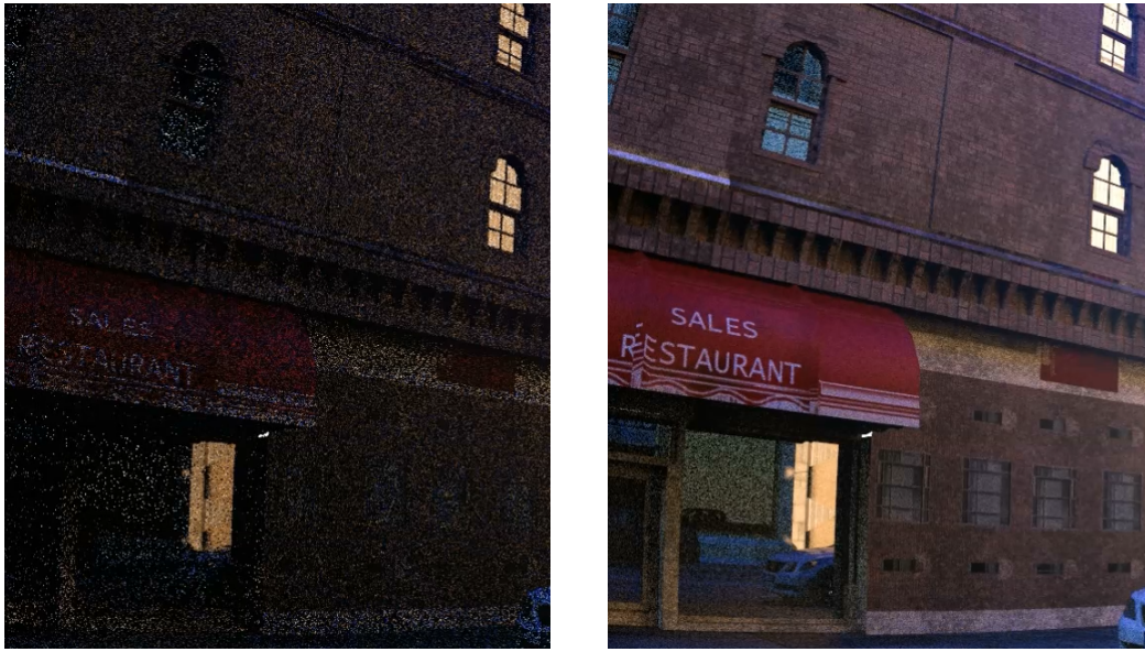
Figure 5.4.2: Screen captures of a video demonstrating the Brigade 3 path tracing engine, originating from http://raytracey.blogspot.com/2013/10/brigade-3.html . The left image shows the path tracing result produced in one frame. The right image displays the image generated after two seconds.
