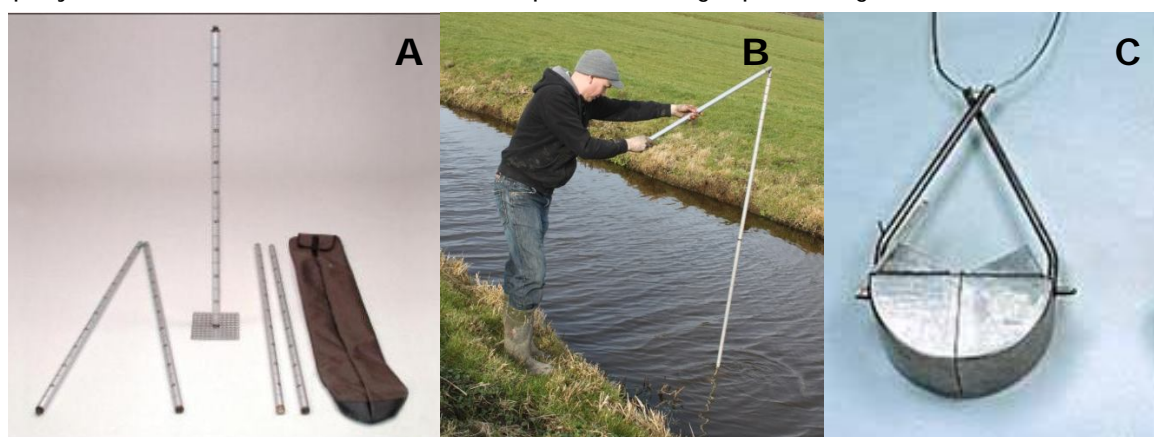
Figure 17: Fieldwork equipment: A) Measuring rod, B) Use of measuring rod and C) Sediment grabber.
