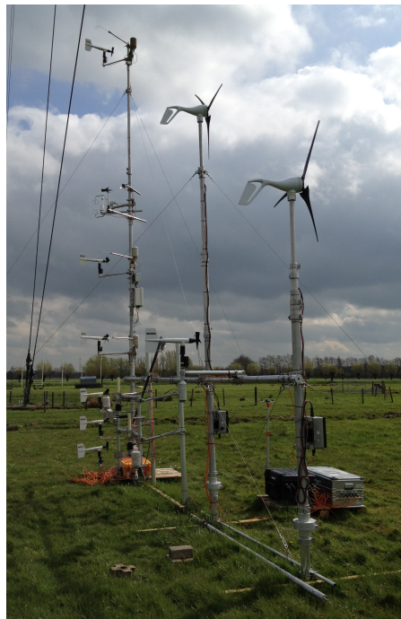
Figure 7.1: Snowdrift measurement setup at a test location in Cabauw.
