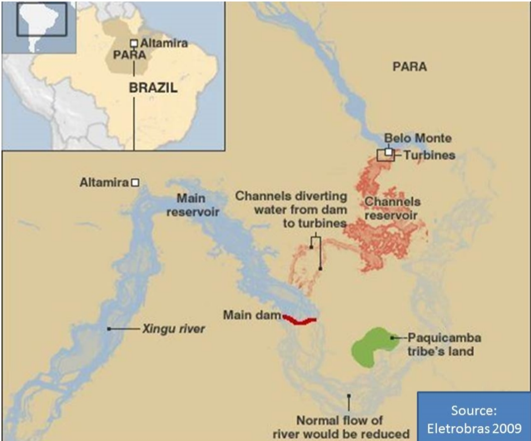
Figure 4, Belo Monte dam ( Eletrobras 2009, adapted).
