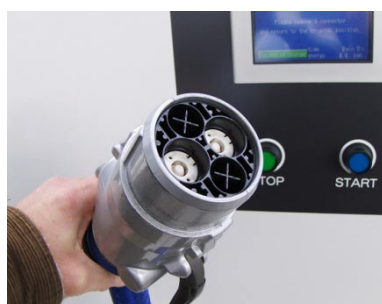
Figure 7. The CHAdeMO plug
