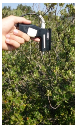
Figure 3. ASD FieldSpec FR operative scales: 25° optic, leaf clip.
