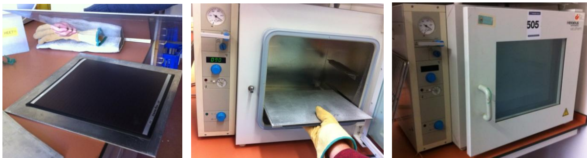
FIGURE 35, MODULE PLACED BETWEEN TWO PLATES IN THE OVEN AT THREE TEMPERATURES: 60, 90 AND 120 °C
