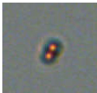
(d) Optical microscope image of a single hematite etched particle (HC1_s2_e2). The particle is more orange, and is smaller than in (b).
