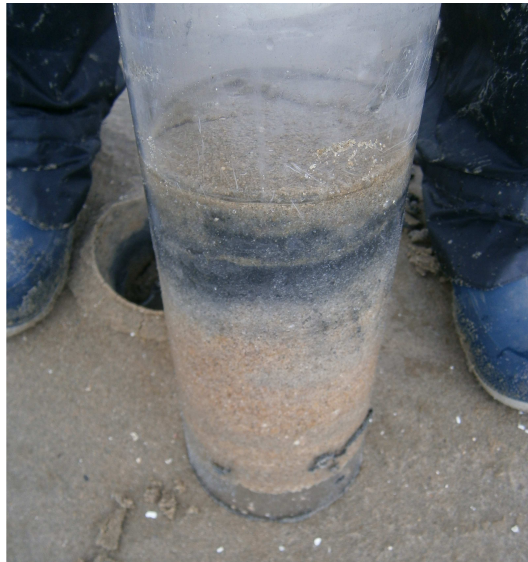
Figure 5.6: The different Sand Motor sand colors. The brown at the bottom of the core is iron oxide, the grey and brownish sand is the normal sand color. The dark grey sand is organic matter (Pit, 2013).
