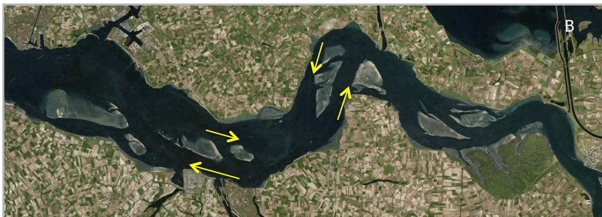
Figure 2.4: (A) Ebb- and flood-tidal channels and bar areas in the Western Scheldt (bathymetry, 2002) (Swinkels et al. 2009). (B) View of Westerschelde with ebb- and flood-dominated channels in yellow with bars inbetween (Bing maps, assessed on April 2013).
