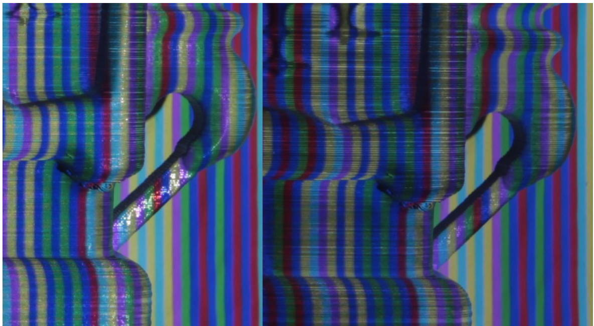
Figure 4.4: Images taken with polarized light. Left; filter at 0 degrees. Right: Filter at 90 degrees.
