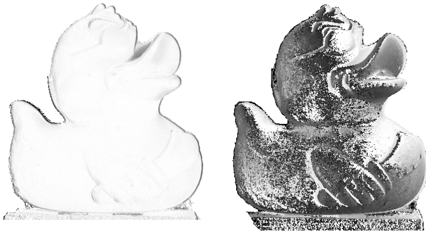
Figure 3.7: Degree of Polarization and Phase of a rubber duck. Left: Degree of polarization. Dark areas indicate a higher DOP. Right: Phase
