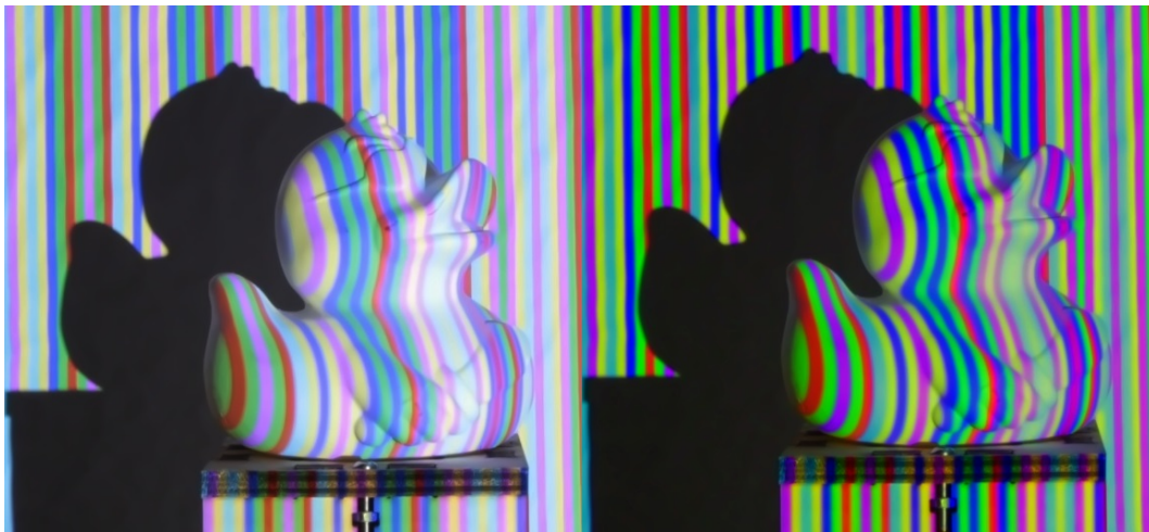
Figure 3.3: Before and after color crosstalk removal; Original pattern.
