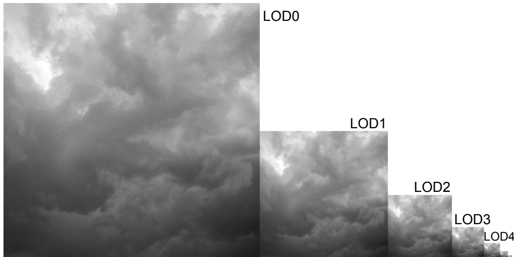
Figure 3.18: Mipmap pyramid of a cloud texture, from 512 \times 512 all the way down to 1 \times 1 . The LOD is shown for the original image (LOD0) and the first three mipmaps (LOD1 through LOD4). © Ilya Khamushkin.
