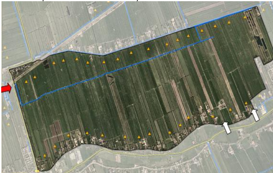
Figure 18: WFD statuses of nutrients and macrophytes in WFD water bodies and ditches in the area Hekendorp. The red arrow indicates a pumping station. The white arrows indicate inlet devices
