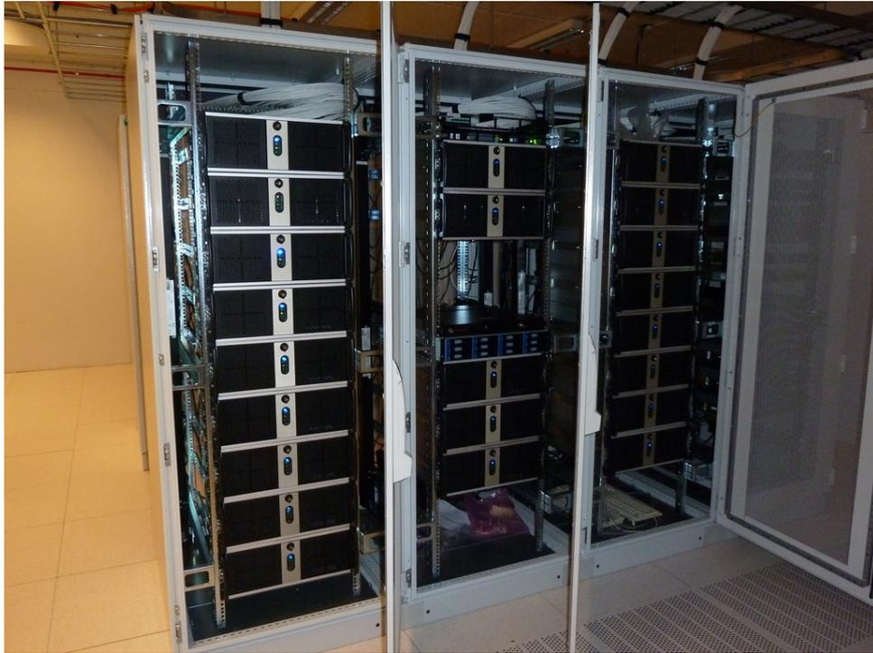
Figure 4.1: The Little Green Machine in Leiden. It contains 20 nodes with each two graphics cards [34].
