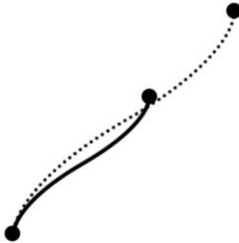
Fig. 3.1: This figure shows the change in the path when a motion is being scaled. The full line represents the motion before scaling and the dotted line represents the motion after scaling.
