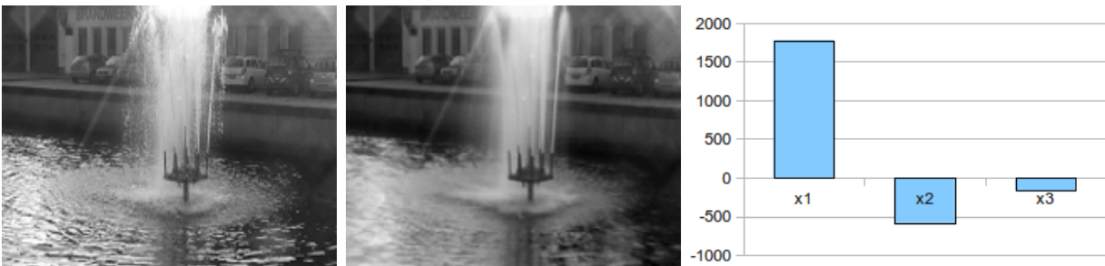
(c) Resp. example video frame, low rank approximation, and weight of each eigenimage in the low rank approximation.
