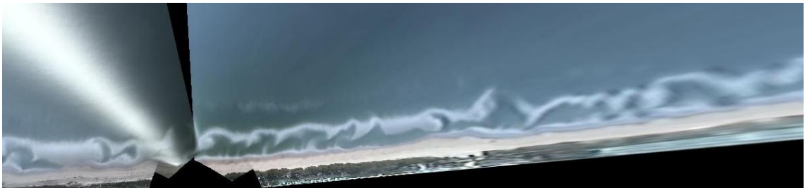
Figure 1.2: Example of a time-exposure image taken on the 4th of August 1999 by the ARGUS system at the Gold Coast, Australia
