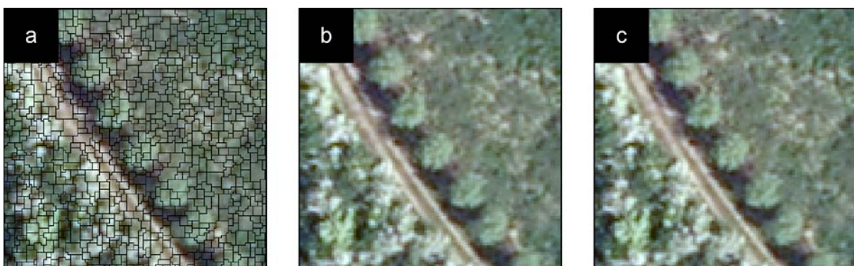
Figure 13: Example of bottom-up segmentation methods: (a) multiresolution segmentation. (b) multi-threshold segmentation. (c) spectral difference segmentation.
