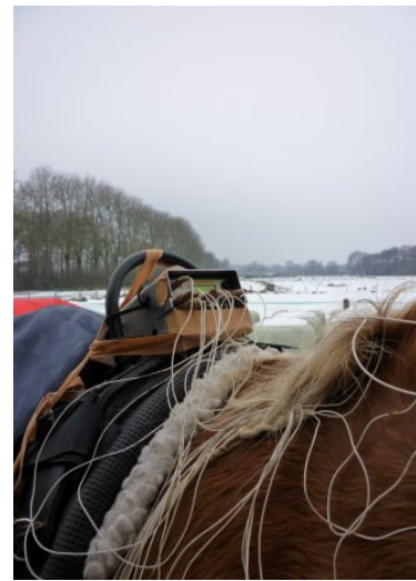
Photo.2 'Porti-5' recording system was attached underneath a metal roll-band on top of a girdle.
