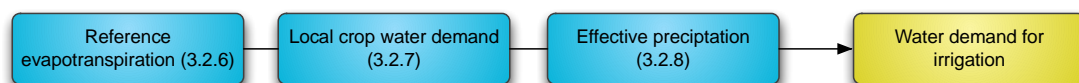
Figure 6: Schematic overview of the methodology of Heibloem and Brouwer (1986) to calculate water demand of irrigated crops
