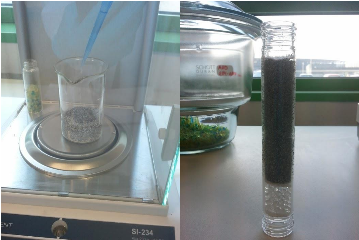
Figure 4.5: Left: Beaker with approximately 40 grams of slag material being wetted with UP water up to the required L/S ratio on the digital balance, before mixing. Right: Detail of the column before the start of the experiment. With starting from below: one filter, a layer of glass beads, 2 filters, the wetted material, 1 filter.
