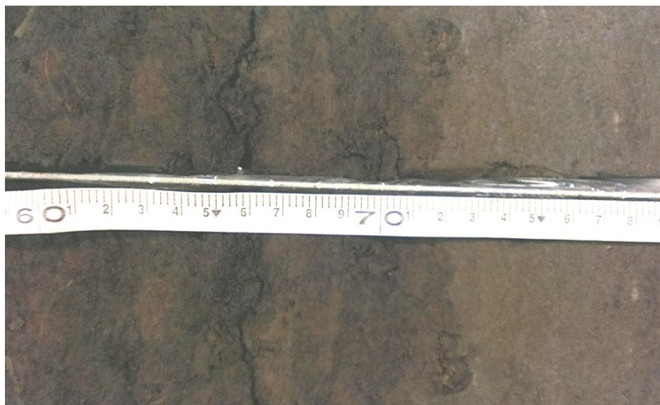
Figure 14. Houterhof 2 core with sharp transition between peat infill and sandy base at about 72 cm. Base of the channel to the right.
