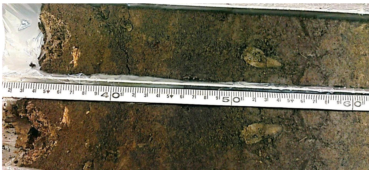
Figure 10. Transition of oxidized peat layer towards clayey peat. Base of the channel to the right.
