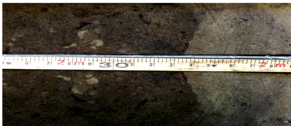
Figure 17. The lowermost part of the Katerhof core (239-225 cm depth), showing the sharp transition between fine sands (with small silt and clay intervals) and sandy gyttja. Base of the channel to the right.
