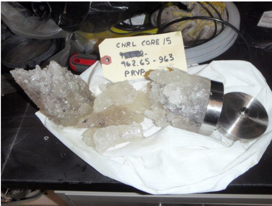
Photograph 5. Failure in Creep – Prairie Evaporite
