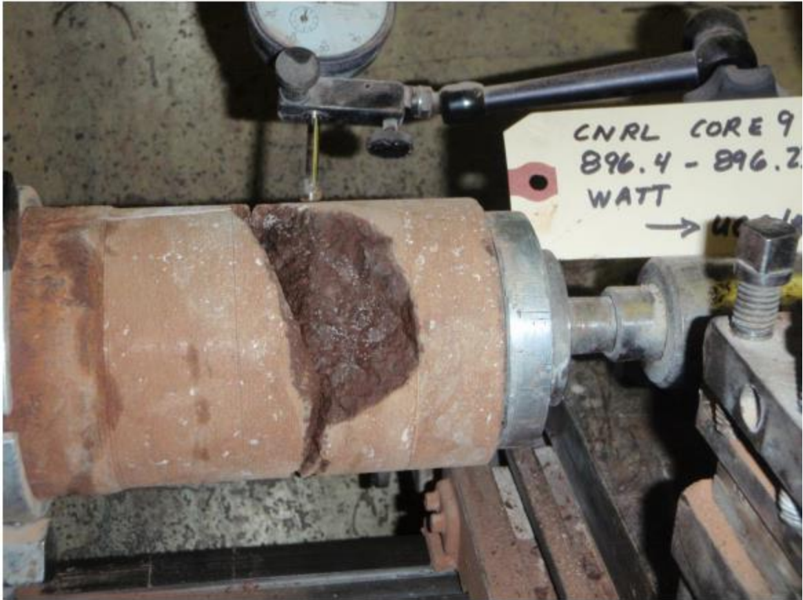
Figure 17. Failure of core sample while lathing.
