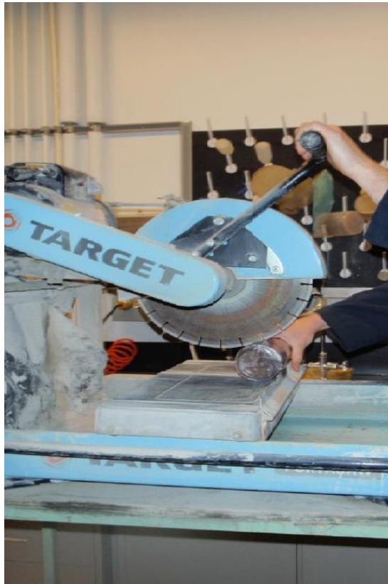
Figure 16. Cutting perpendicular ends.
