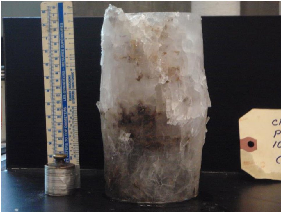
Photograph4. Failure in Constant Mean Compression Test – Prairie Evaporite
