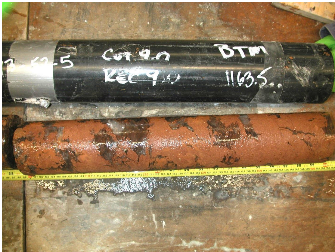
Figure 29. Clay content of the Cold Lake Formation near the interface with the Ernestina Lake Formation
