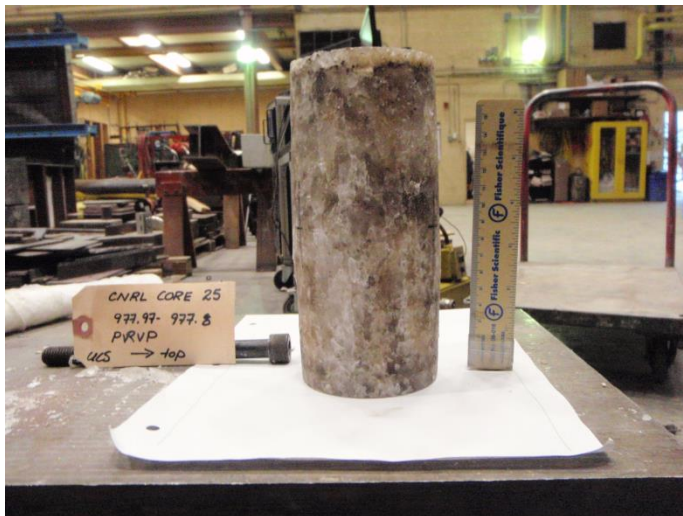
Photograph 3. Failure in Unconfined Compression – Prairie Evaporite
