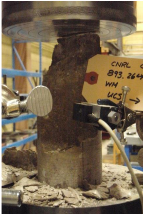
Photograph 1. Failure in Unconfined Compression – Watt Mountain
