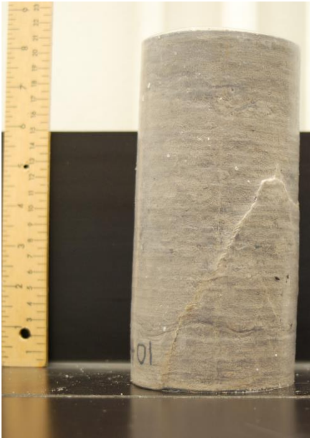
Photograph 7. Failure in Standard Triaxial Compression – Keg River
