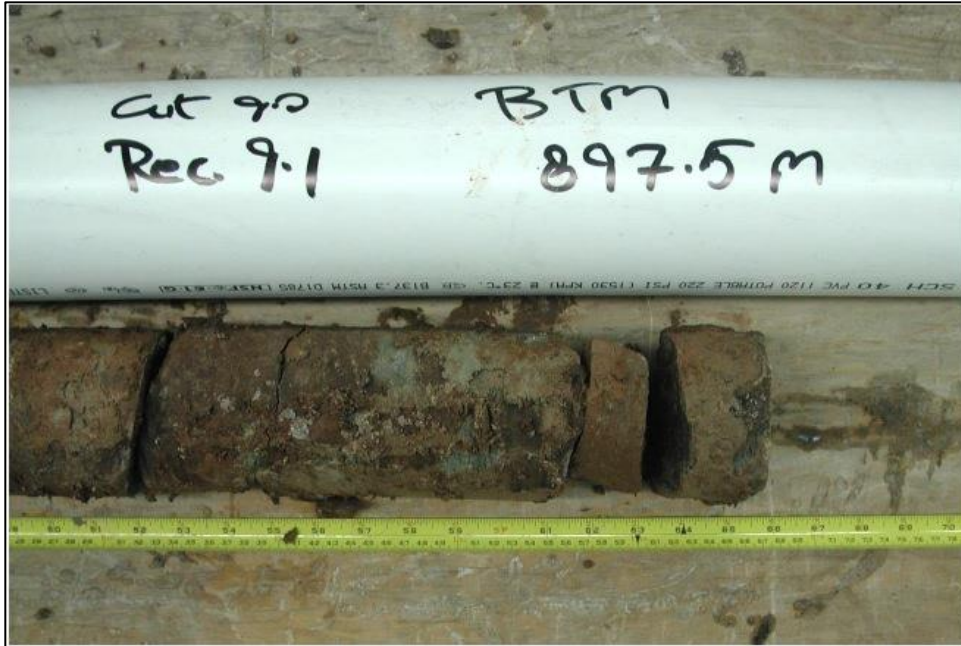
Figure 24. Typical weathered core material from the Watt Mountain Formation
