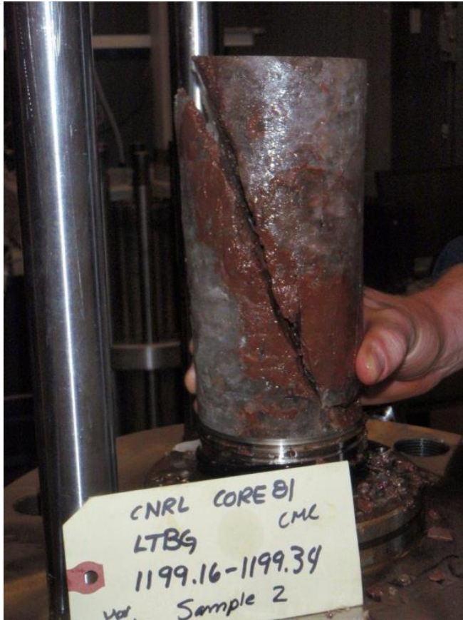
Photograph 12. Failure in Constant Mean Compression Test - Lotsberg
