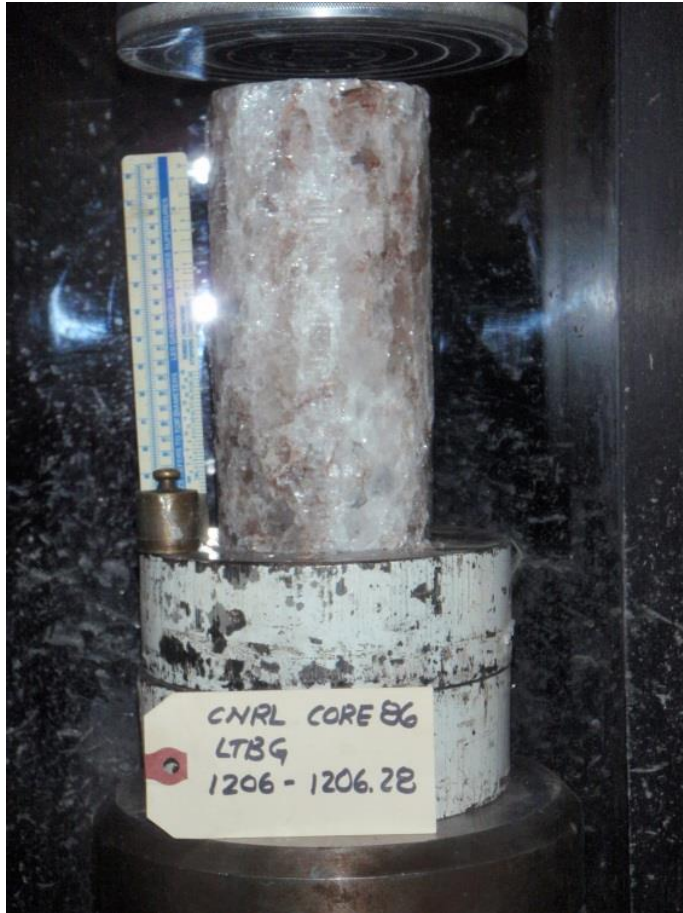
Photograph 11. Failure in Unconfined Compression - - Lotsberg
