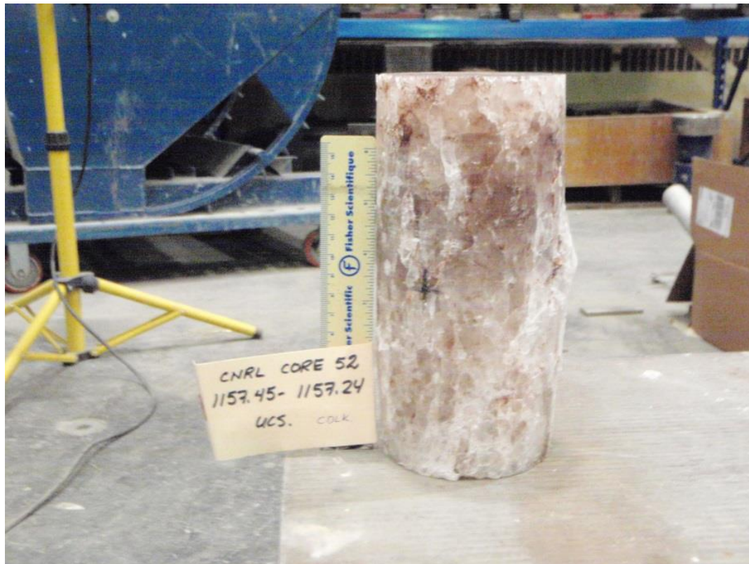
Photograph 8. Failure in Unconfined Compression Test – Cold Lake
