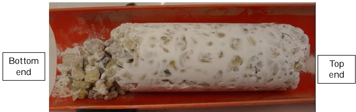
Figure 2.4 Cementation of column with Ecogrout process (Van der Star 2012)
