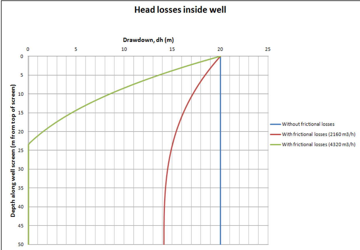
Fig. 28. By simulation, this could be a good portrait of what goes on during the process of surging. Because high discharges during surging, the hydraulic gradient in the top of the aquifer can be much bigger than it is in the lowest part. Head losses are bigger in the upper part. In reality the assumed linear cumulative discharge cannot be reality, where varying head losses and evenly distributed water intakes contradict one another.
