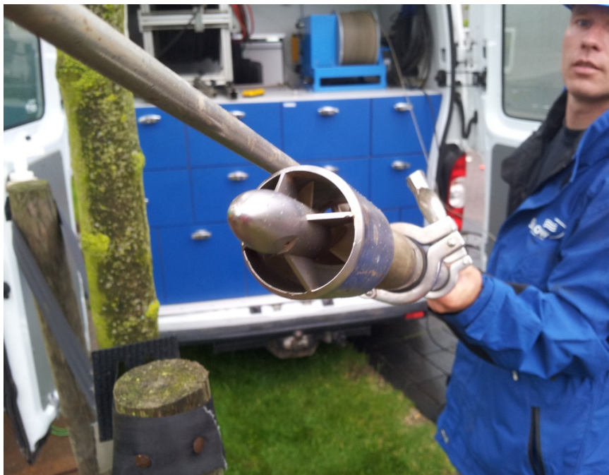
Fig. 42. Impeller flowmeter used by Q-flow, Rabobank Utrecht project.
