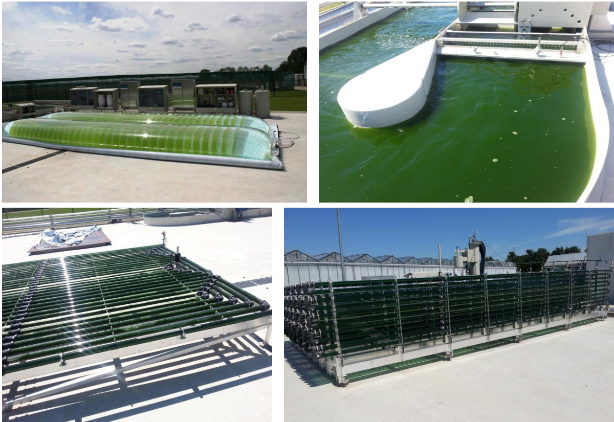
Figure 5 - Microalgae cultivation systems: 1 - Flat plate in plastic bag, 2 - Open raceway pond, 3 - Horizontal tubular PBR, 4 - Vertically stacked horizontal tubular PBR (all pictures are taken at AlgaeParc Wageningen).
