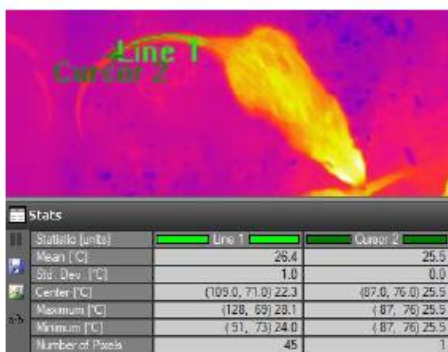
Figure 4 Measuring mid-tail temperature with a bendable line ROI and a 1-pixel cursor ROI in the FLIR ResearchIR program.
