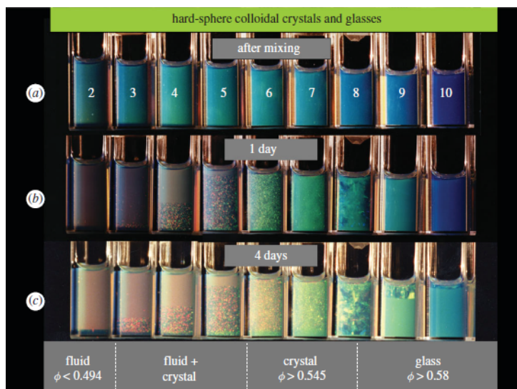
Figure 2.2: The phase behaviour of colloidal crystals, as function of their volume fraction. In relatively concentrated sample, crystal and glass formation is observed.
