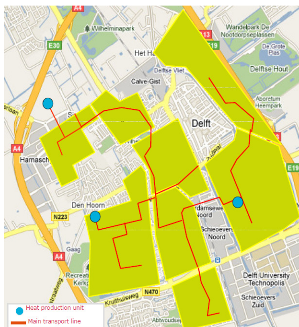
Figure 8: District heating network Delft
