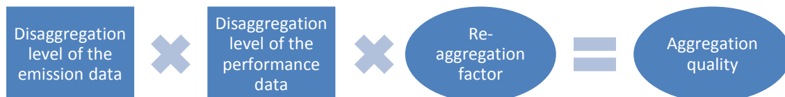
Figure 4.2: The formula used for the aggregation quality. The square form indicates a value based on one of the parameters and the circle indicates a value based on the combined intensity indicator.
