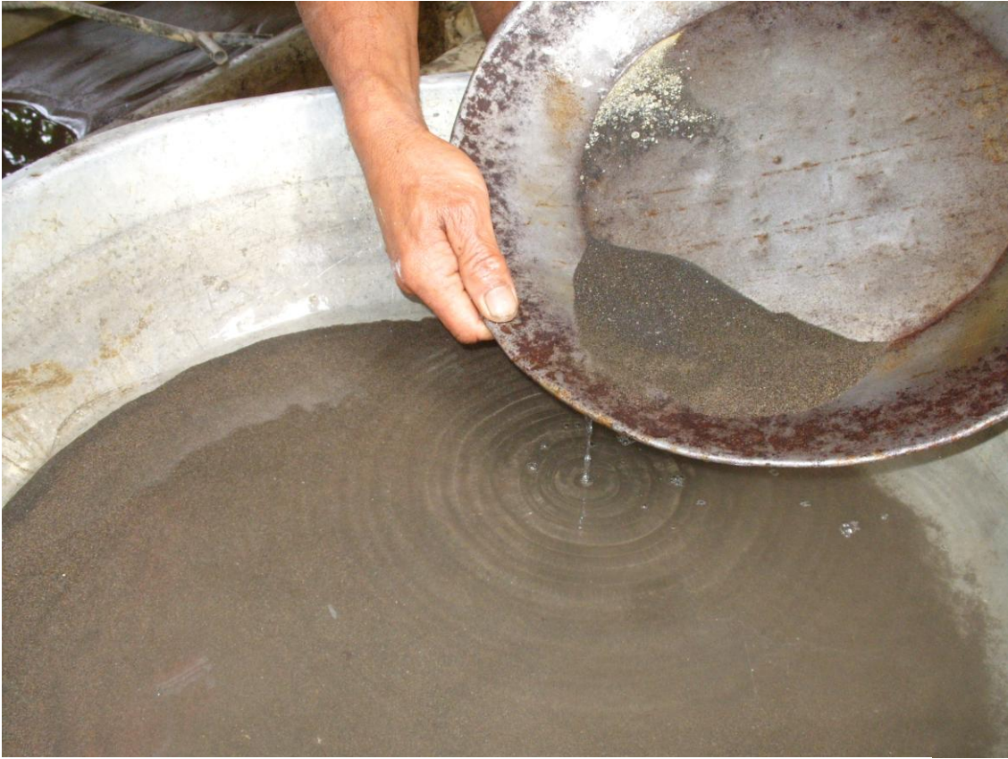
Photograph 13: gold panning. Testing if the naba contains gold by gravity separation, using water and a sample pan.
