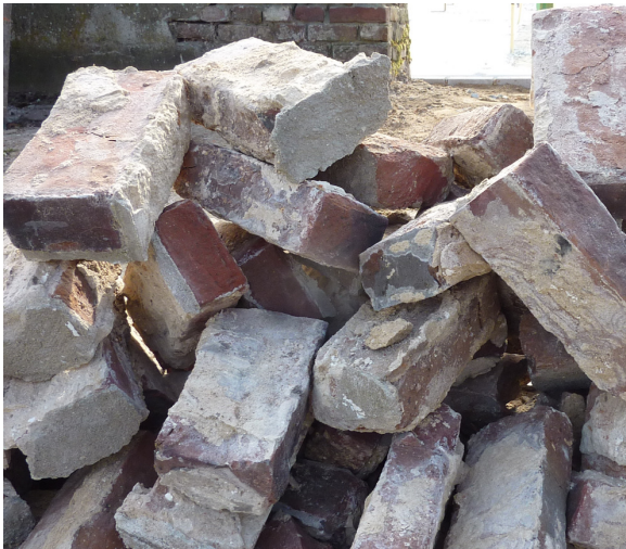
Figure 3.2 – ceramic clay bricks with mortar. The brick can be re-used in case the mortar is removed.
