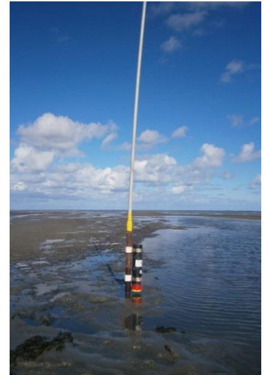
Figure 6-10 One pressure sensor, attached to a steel pole.
