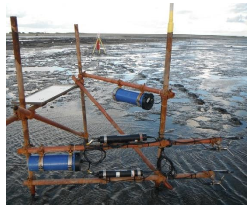
Figure 6-11 The frame and two ADV's, placed in front of the mussel bed
