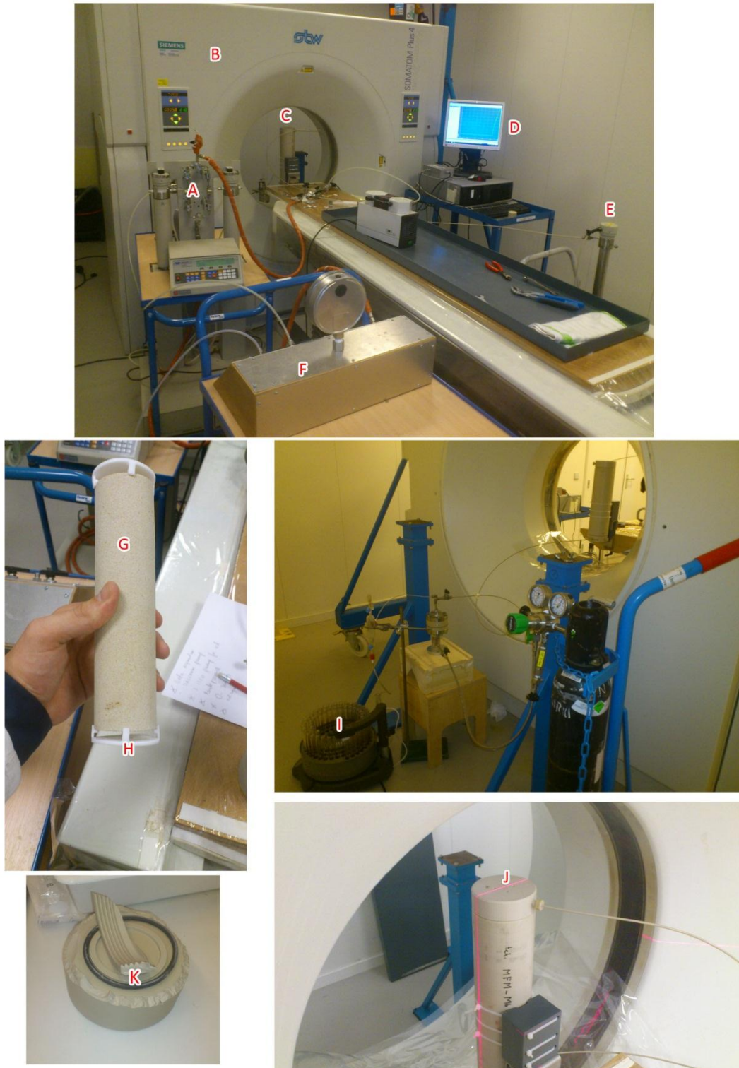
Figure 3 Set-up 2: A) Double ISCO-pump for CO 2 injection B) CT-Scanner C) Core holder D) Data acquisition E) ISCO-pump for oil injection F) Gas booster G) Bentheimer sandstone core H) Teflon placer I) Fraction Collector J) CT-scan X-ray at the middle of the core K) Core holder failure
