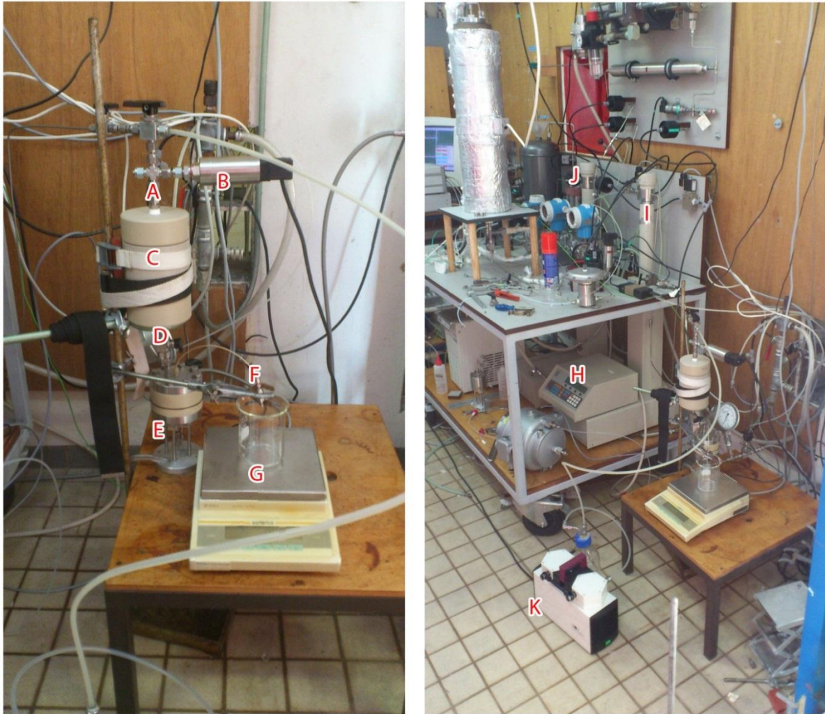
Figure 2 Set up 1 A) Injection line B) Pressure transducer C) Core holder D) Production Line E) Back-pressure regulator F) Separator G) Balance H) Isco Pump controller I) Double Isco Pump J) Gas Injection K) Vacuum pump
