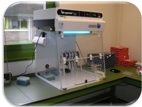
Figure 14: The PCR area where the PCR mix is made is extra clean. CVI©
