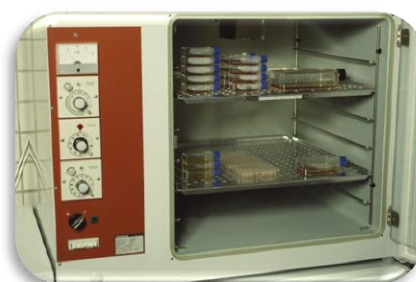
Figure 5: An incubator for cell culture and virus culture. CVI©
