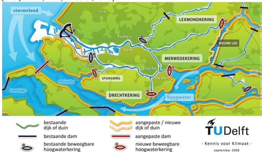
Figure 17: The “Afsluitbaar Open Rijnmond” concept from Ties Rijcken, TU Delft and HKV lijn in water (from Hoss, 2011).
