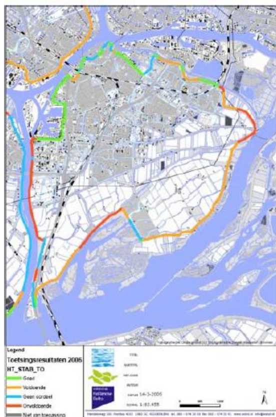
Figure 16: The results of the 5 year review of the embankments by the water boards of 2006 from Van Herk et al. (2011).
