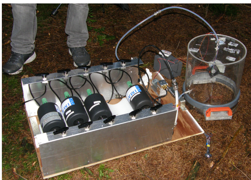
Fig. 2.2 Samper structure. The chamber is 22.8 L and each flask is 1 L in volume.
