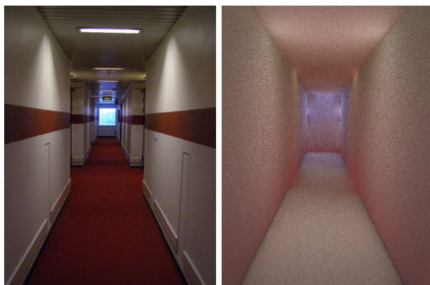
Figure 5.3: Irradiance map. At every pixel of the room, the irradiance is computed by sampling the hemisphere around that point in three dimensional space. This gives a representation of the amount of indirect light received by the point visible at that pixel. For example, the floor receives most light from the walls, yielding white, while the lower part of the walls are more red because of the carpet. The noise can be reduced by increasing render time.
