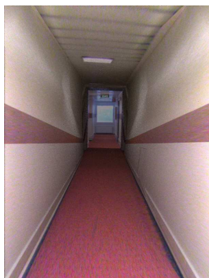
Figure 5.4: Incorrect texture mapping obtained by using the input image directly as a uv -map. Note: the colors in this image are inaccurate, because of an unrelated problem with texture gamma at the time, which is explained in Section 5.1.4.
